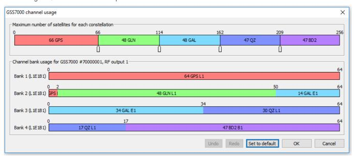
Figure 6 Dynamic channel allocation control concept
