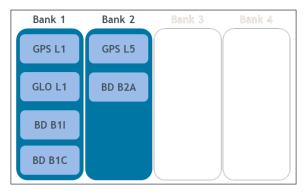
Figure 8 Dual-frequency, 3-constellation system
