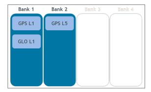
Figure 7 Dual-frequency, 2-constellation system
