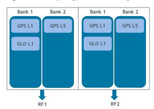
Figure 10 Dual-freq, 2-constellation 2RF system
