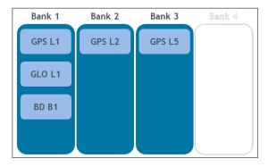
Figure 9 Triple-frequency, 3-constellation system
